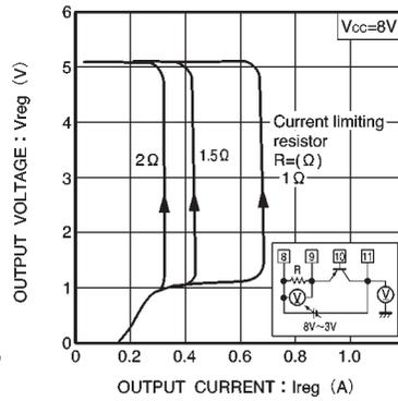
Fig.9 Regulator output voltage vs. regulator output current
