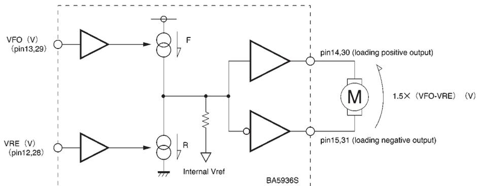
When  $V_{FO} < V_F$  (approx. 0.6V),  $V_{FO} = 0V$
