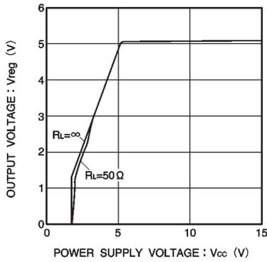
Fig.8 Regulator output voltage vs. power supply voltage
