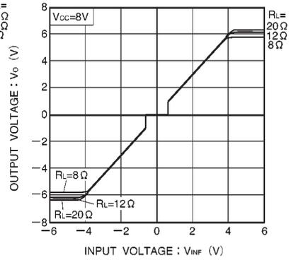
Fig.7 Loading driver I/O characteristics (channels 3 and 6)
