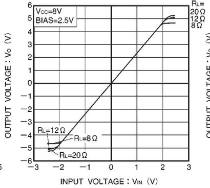
Fig.6 Driver I/O characteristics (channels 1, 2, 4, and 5)
